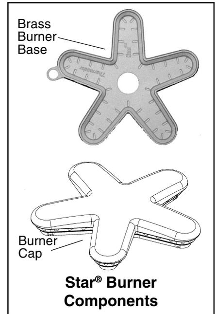
Each burner has its own electronic igniter that sparks when the burner is turned on. Each burner should light in 4 seconds or less. If a burner does not light, check to see that the cap is positioned correctly on the base.
